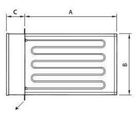
Mounting flange; the electrical connection box outside the air handling unit.
