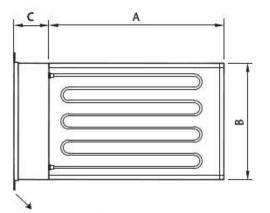
Mounting flange; the electrical connection box inside the air handling unit.
