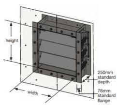
Min. Size\* 200mm x 200mm Max. Single Section\* 1220mm x 1524mm (see graph for blast pressure limitations). Max. Multi-Section\* 2440mm x 1524mm (subject to blast pressure limitations)
