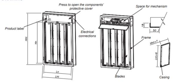
The servomotors are supplied for 24 V operation 230 V operation available on request. GMCAIR incorporates motors from different manufacturers (Belimo, Siemens, etc.).
