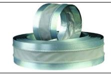
Flexible Connector prevents vibration and noise to transfer the galvanized duct which carries air in heating ventilation systems. The material which is placed between two galvanized sheet is locked with multi lock system. Never seperates each other.
